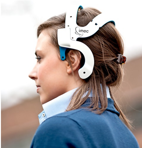
Fig. 3: Prototype for EEG-sensing headset.
